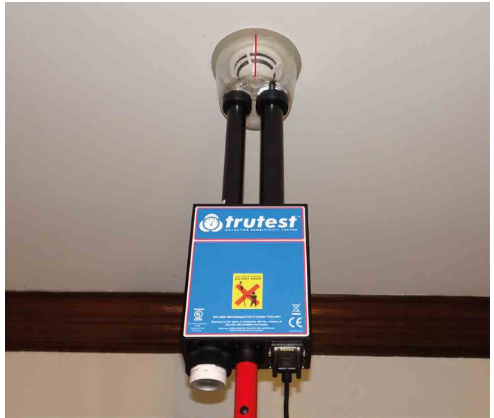
Figure 13: Trutest being used to test a commercial smoke detector
