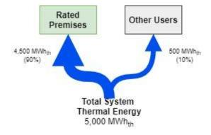
Figure 4.4: Determine percentage of total shared chilled water system thermal energy allocated to rated premises
