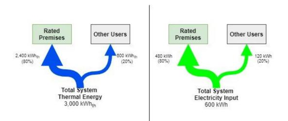
Figure 4.3: Example – allocating energy inputs to thermal energy outputs on an hourly basis.
