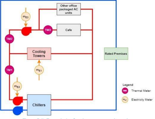
Figure B.7: Example 2 – Condenser water schematic
