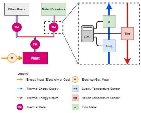
Figure 4.1: Typical thermal energy metering configuration
