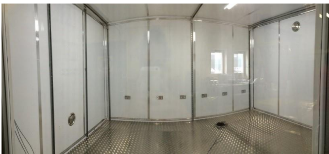
IAQ sensor and monitor performance has been investigated in one of BRE's room-sized environmental chambers - the 30m 3 chamber pictured here.
