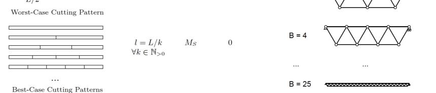
Worst and best cutting patterns for cutting a set of identical structural elements of length *l* from inventory elements all of some length L.  $M_s$ : Structural mass.  $M_t$ : Inventory mass consumed.  $M_w$ : Offcut waste mass produced.
