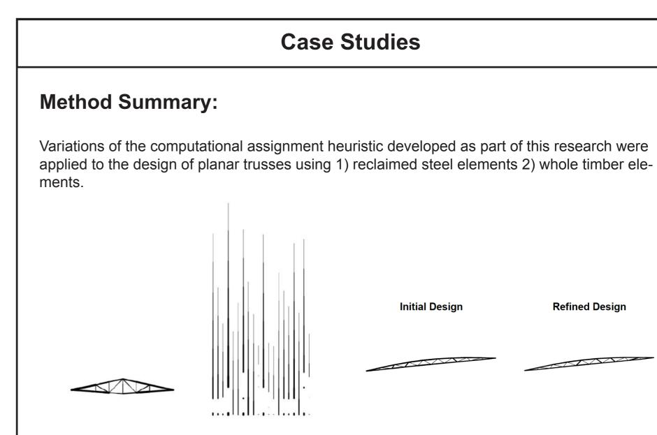
Assignment of an inventory of whole timber elements to a planar whole timber truss subject to member ULS constraints. Shown: random pre-sorting of structural locations, pre-sorting of inventory elements by base diameter. within serviceability limits.
