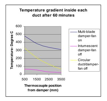
Figure 15. Temperature gradient inside each duct at 60 minutes
