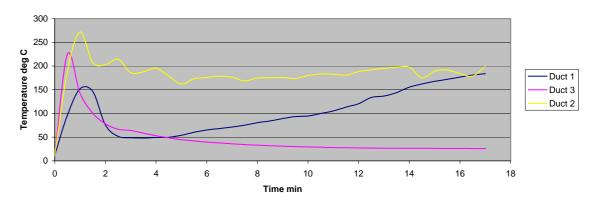
Figure 13. Temperatures 500mm from damper in first 17 minutes of test
