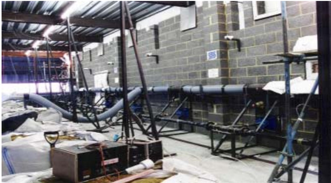
Figure B5 Gas fired furnace – Plane frame test
