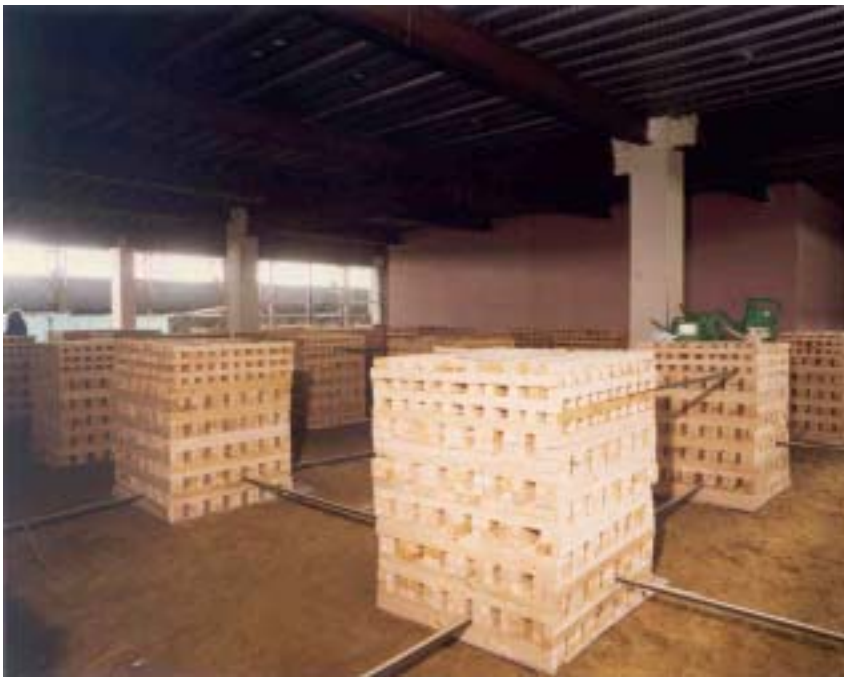
Figure B18 crib layout BRE large compartment test
