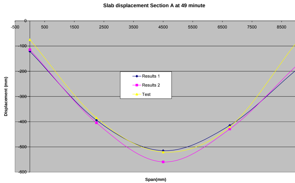
Figure E26: Slab displacement on section at 49 minutes
