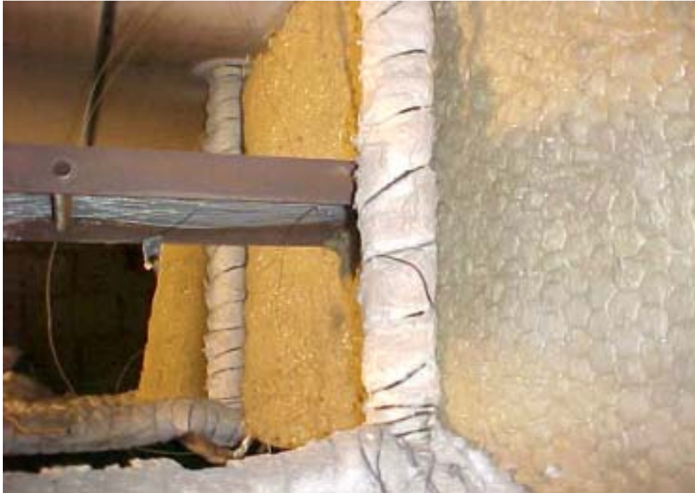
Photograph B5. Thermocouples on the exposed side to the burner.
