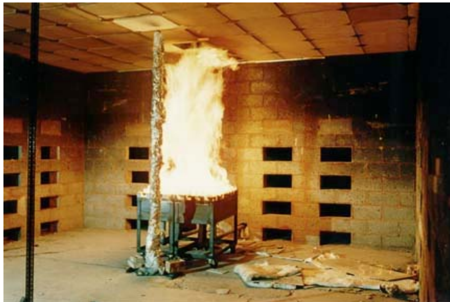
Photograph B2. 1 MW gas burner with flames entering ceiling void
