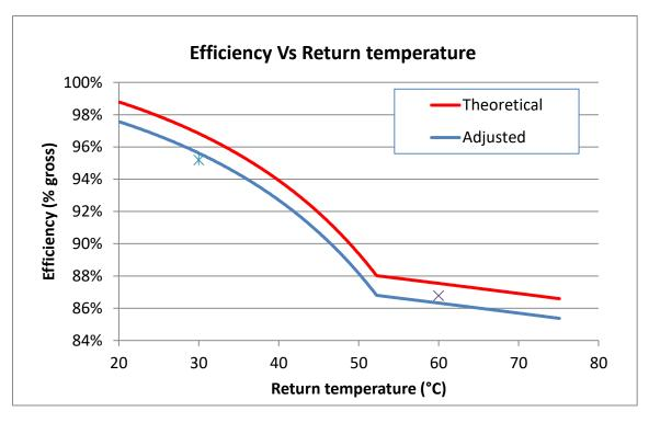
Figure 5 - Gas boiler efficiency relationship for theoretical and example boiler
