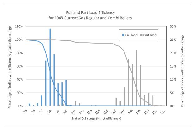
Figure 7 - Gas boiler efficiency data held in PCDB (January 2016)
