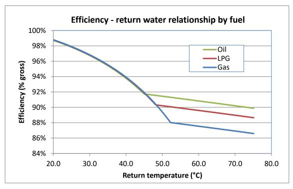
Figure 2 - Boiler efficiency - return water temperature relationship by fuel
