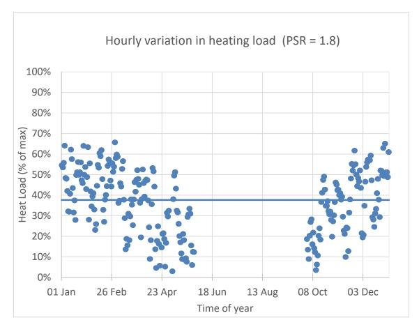
Figure 3 - Variation of heating load fraction (Fload\_inter)
